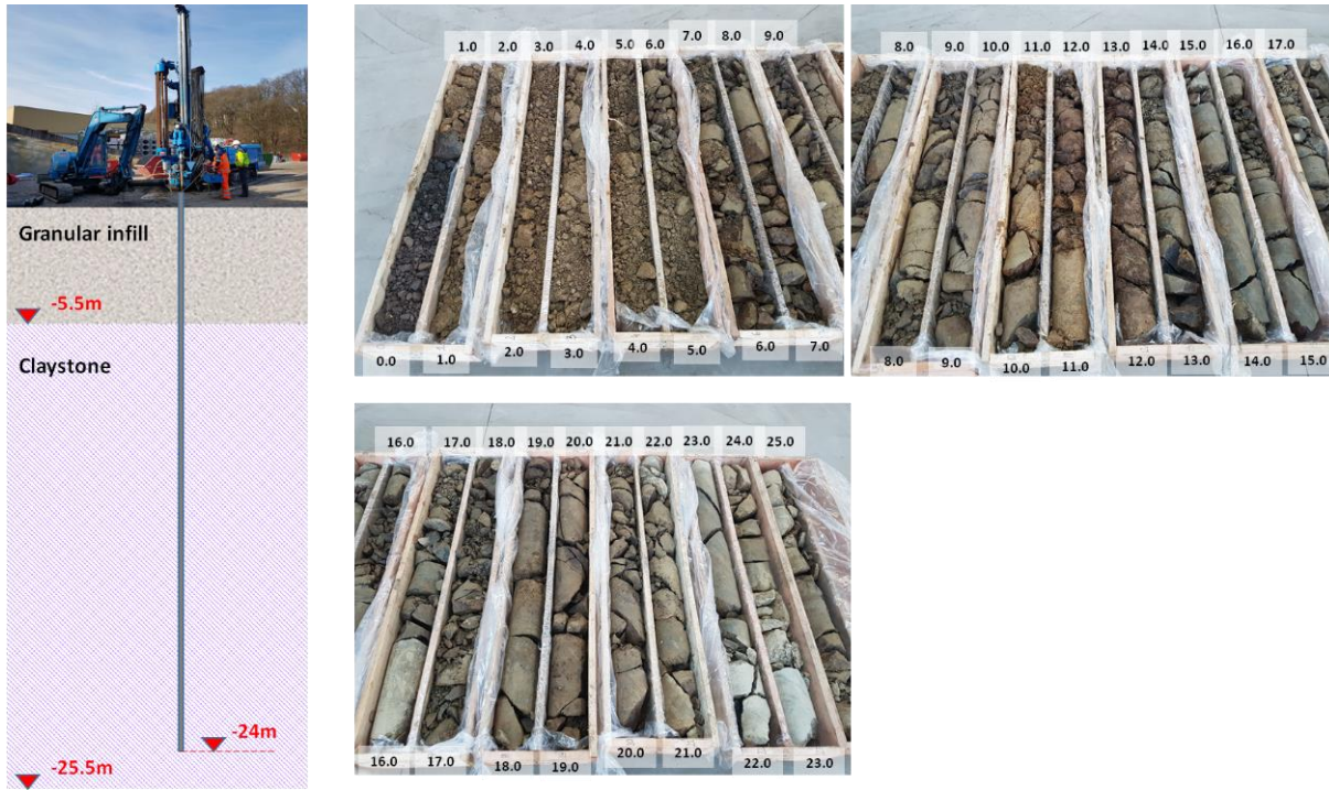
Fig. 5 Ground conditions at the trial site
